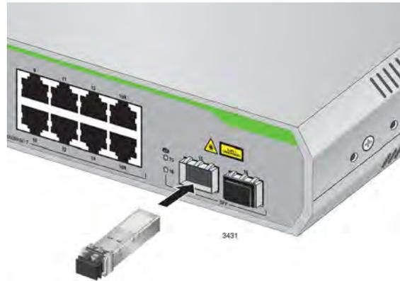
Figure 13. Inserting the SFP
