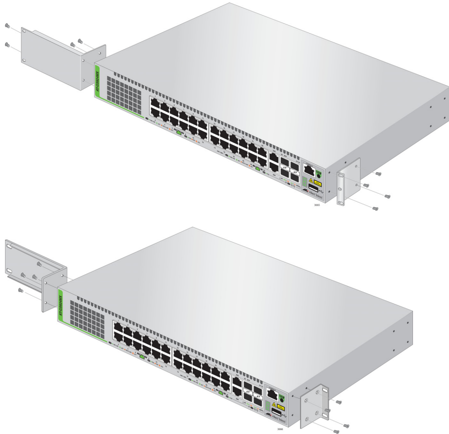
Figure 19. Installing Brackets on the AT-GS924MX Switch
