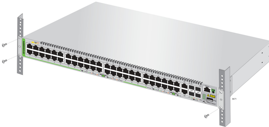
Figure 22. Mounting the Switch in an Equipment Rack
