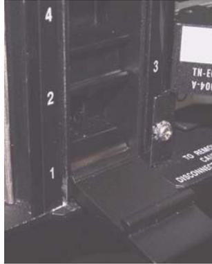
**FIGURE 1-6 FM7 fully inserted with lock-latch open**
