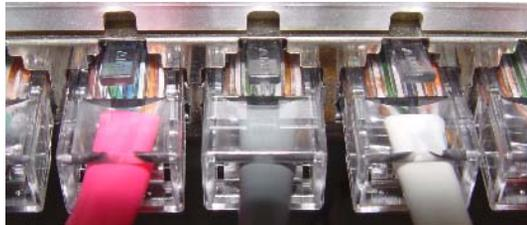
FIGURE 1-18 FE10 data cable connectors
