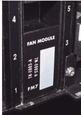
**FIGURE 1-7 FM7 inserted with lock-latch closed**
