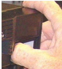
FIGURE 1-8 Curl thumbs behind lock-latches and press release buttons (right side detail)
