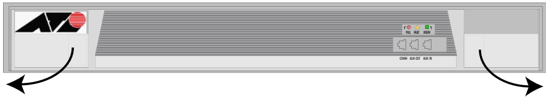
FIGURE 1-7 FAN8, arrows indicate latch opening
