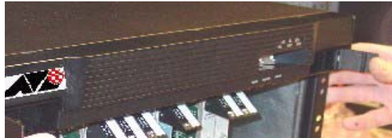
FIGURE 1-11 Swing the lock-latches in to close them
