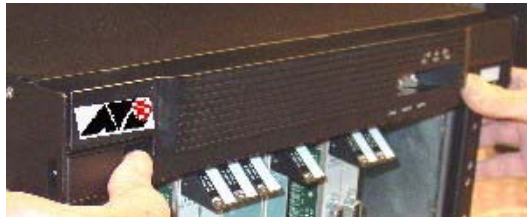
FIGURE 1-12 Close the lock-latch
