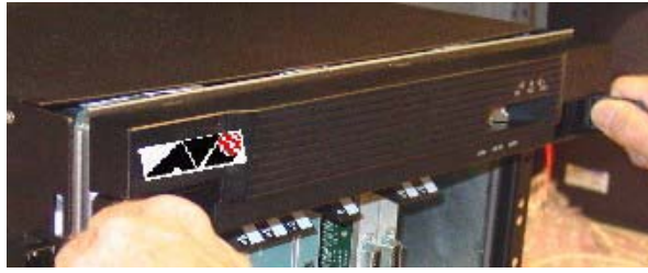
FIGURE 1-10 Slide the FAN8 into the chassis
