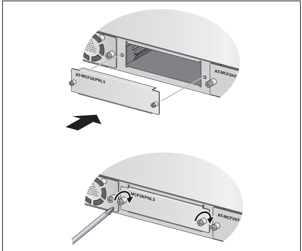
Figure 92. Installing the AT-MCF2KPNL3 Slot Cover on the Management Slot
