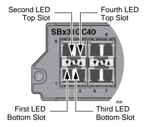
Figure 23. LEDs for the AT-SBx31GC40 Line Card
