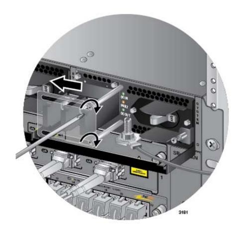
Figure 155. Closing the Plastic Cover
