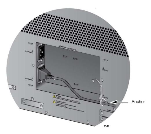
Figure 106. Securing the Power Cord for the AT-SBxPWRSYS1 or AT-SBxPWRSYS2 AC System Power Supply to an Anchor
