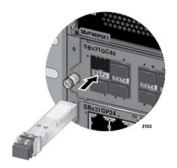
Figure 89. Inserting an SFP or a CSFP Transceiver
