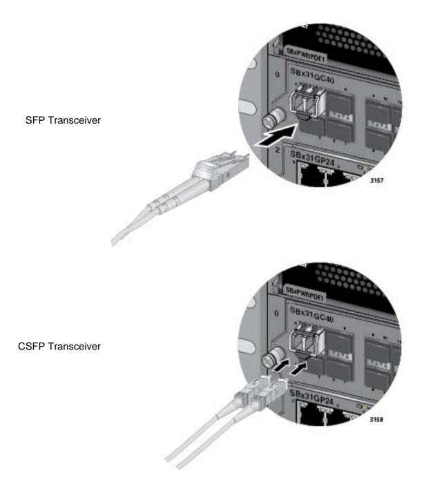
Figure 91. Attaching a Fiber Optic Cable
