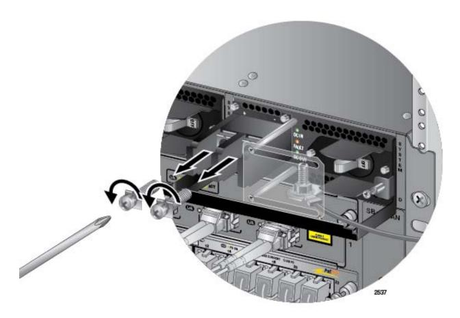
Figure 124. Removing the Terminal Screws
