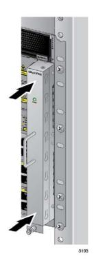
Figure 166. Securing the AT-SBxFAN12 Fan Module on the Backplane Connector
