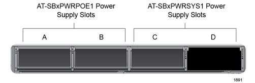
Figure 47. Power Supply Slots
