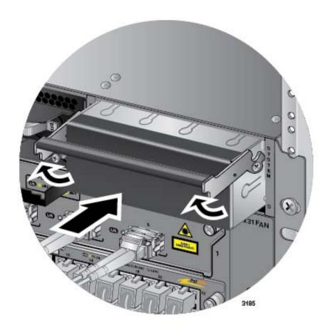
Figure 159. Installing a Blank Power Supply Slot Cover
