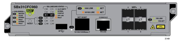
Figure 30. Controller Fabric Cards for the AT-SBx3112 Chassis
