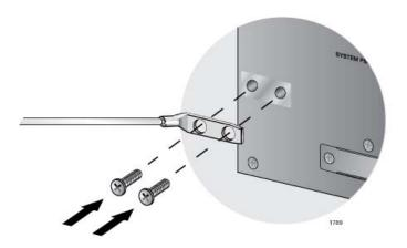
Figure 45. Installing the Grounding Lug and Wire
