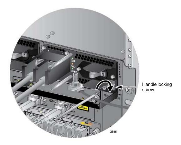
Figure 135. Tightening the Handle Locking Screw
