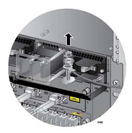
Figure 156. Removing the Grounding Wire
