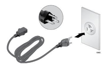
Figure 32. 100 - 125 VAC 125 V NEMA 5-20 Plug and Receptacle
