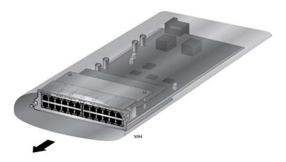
Figure 74. Removing an Ethernet Line Card from an Anti-static Bag
