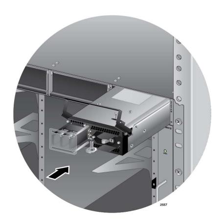
Figure 62. Inserting the AT-SBxPWRSYS1 DC System Power Supply
