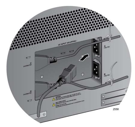
Figure 107. Connecting the AC Power Cord for the AT-SBxPWRPOE1
