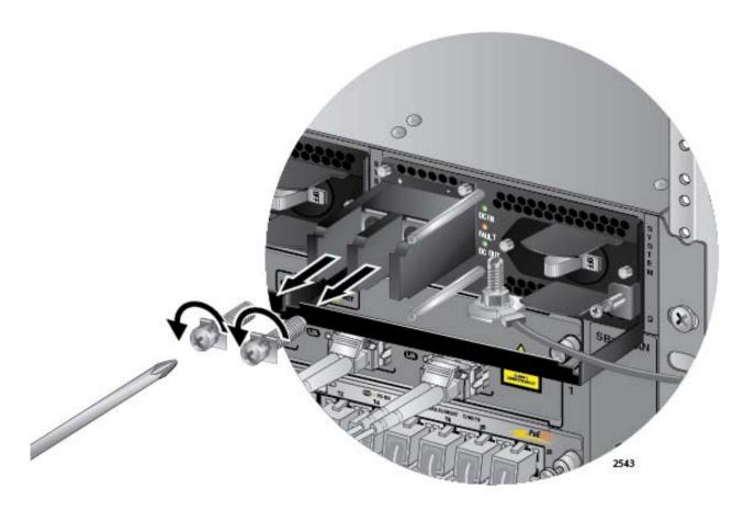
Figure 132. Removing the Terminal Screws
