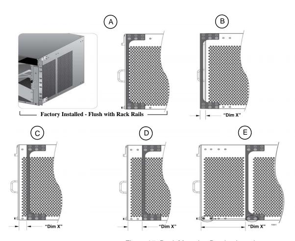
Figure 37. Rack Mounting Bracket Locations
