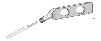
Figure 44. Attaching the Grounding Wire to the Grounding Lug
