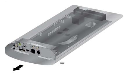
Figure 67. Removing the AT-SBx31CFC Controller Fabric Card from the Anti-static Bag
