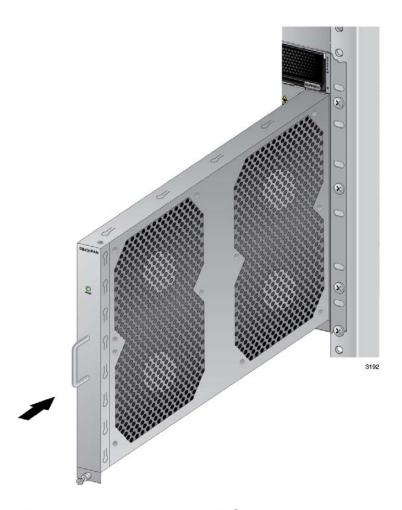
Figure 165. Installing a New AT-SBxFAN12 Fan Module
