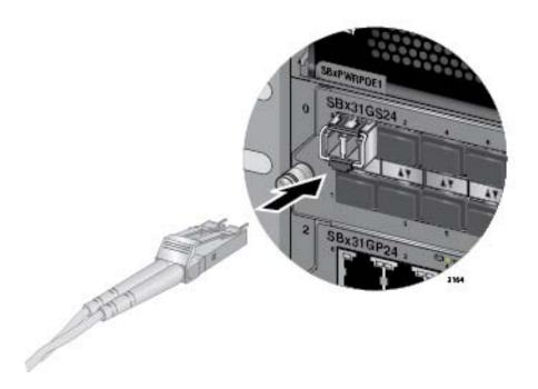
Figure 86. Attaching a Fiber Optic Cable to an SFP Transceiver in the AT-SBx31GS24 Line Card
