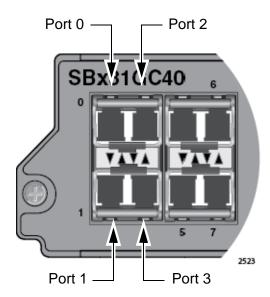
Figure 21. Port Numbers for Slots with CSFP Transceivers
