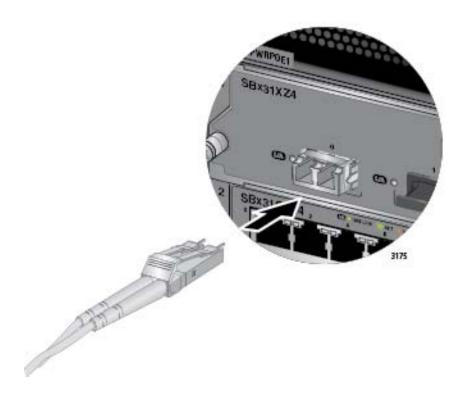
Figure 103. Attaching a Fiber Optic Cable to an XFP Transceiver in the AT-SBx31XZ4 Line Card
