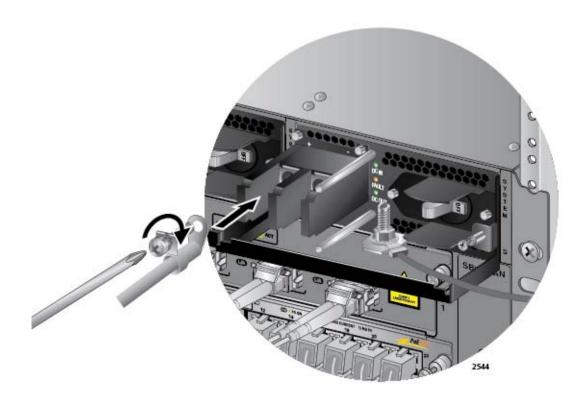
Figure 133. Connecting the Positive (+) Power Wire with a Right Angle Terminal
