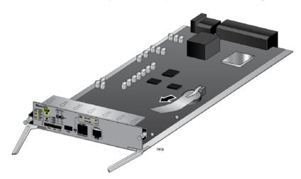
Figure 69. Removing the Battery Insulator
