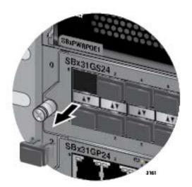
Figure 82. Removing the Dust Cover from an SFP Slot in the AT-SBx31GS24 Line Card
