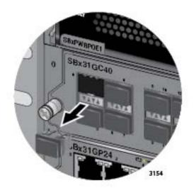
Figure 87. Removing the Dust Cover from a Transceiver Slot on the AT-SBx31GC40 Line Card
