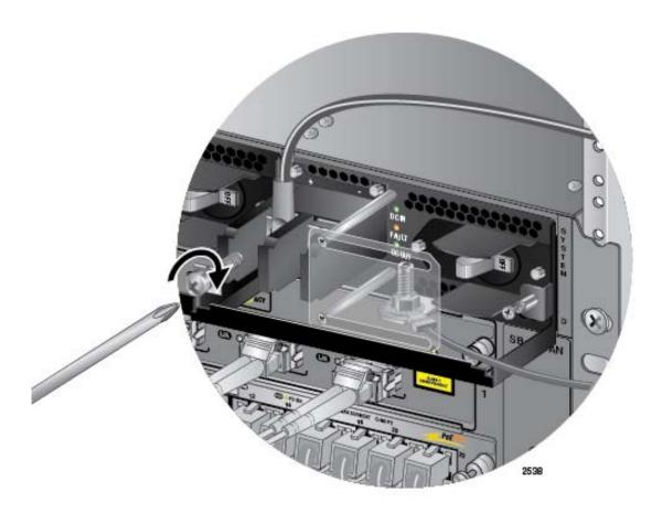
Figure 125. Connecting the Positive (+) Power Wire with a Straight Terminal
