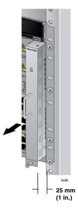
Figure 163. Withdrawing the AT-SBxFAN12 Fan Module 25 mm (1 in.) from the Chassis
