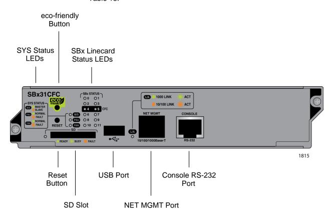
Figure 31. AT-SBx31CFC Controller Fabric Card
