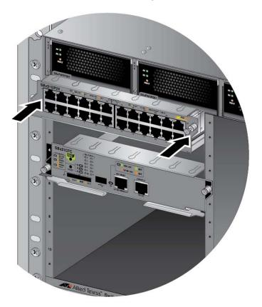
Figure 76. Seating an Ethernet Line Card on the Backplane Connector
