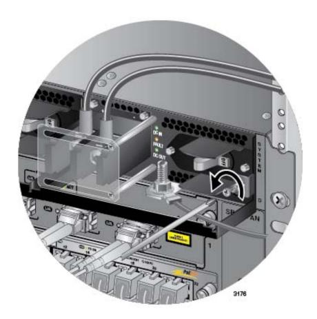
Figure 150. Loosening the Screw on the Locking Handle
