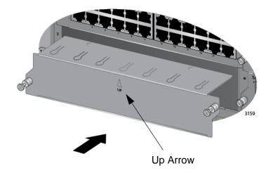
Figure 78. Installing a Blank Slot Cover
