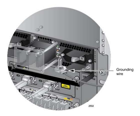
Figure 115. Installing the Grounding Wire
