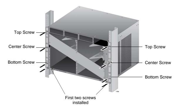
Figure 40. Installing the Rack Mount Screws
