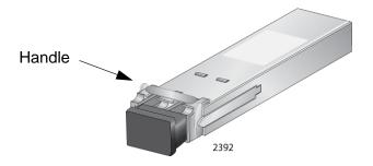
Figure 100. Handle on the XFP Transceiver
