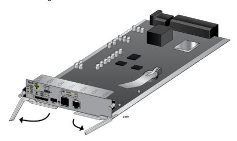
Figure 68. Opening the Locking Handles on the AT-SBx31CFC Controller Fabric Card
