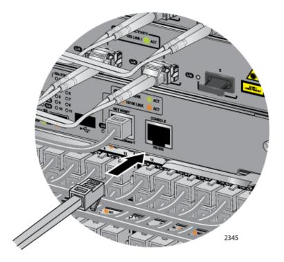
Figure 141. Connecting the Management Cable to the Console RS-232
