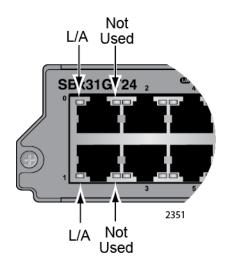
Figure 12. Port LEDs on the AT-SBx31GT24 Line Card
