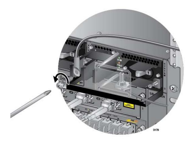
Figure 153. Removing the Positive Lead Wire
