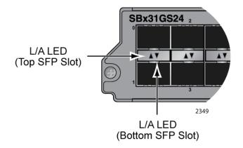
Figure 19. Port LEDs on the AT-SBx31GS24 SFP Line Card
