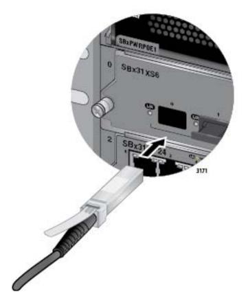
Figure 98. Installing the AT-SP10TW Cable in the AT-SBx31XS6 Line Card
