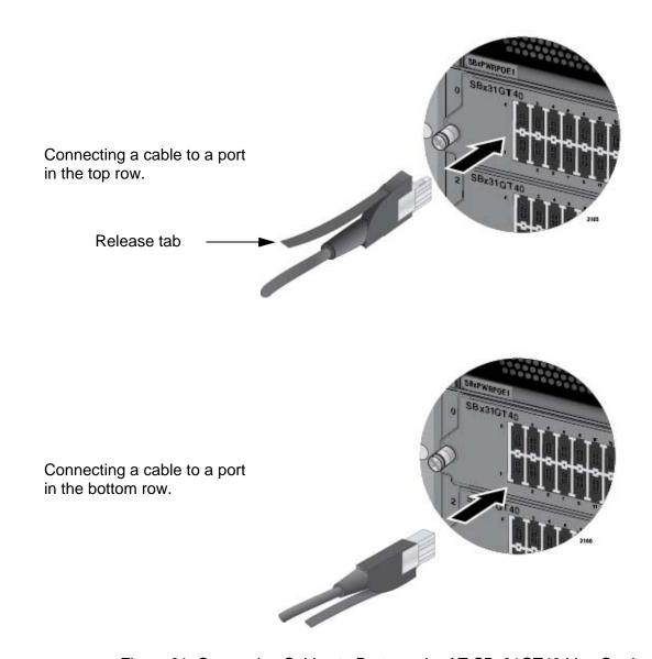
Figure 81. Connecting Cables to Ports on the AT-SBx31GT40 Line Card
