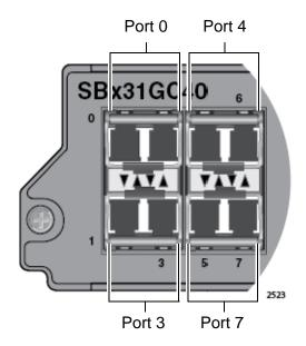
Figure 22. Port Numbers for Slots with Standard SFP Transceivers
