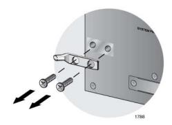
Figure 43. Removing the Grounding Lug
