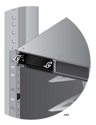
Figure 57. Locking the Handle on the AT-SBxPWRPOE1 AC Power Supply
