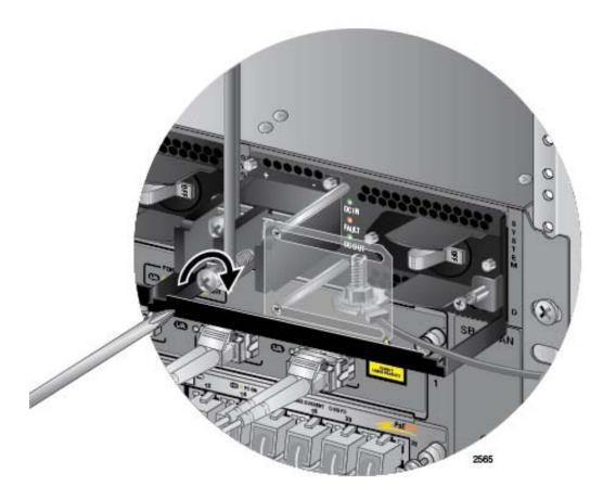
Figure 138. Connecting the Negative Lead Wire
