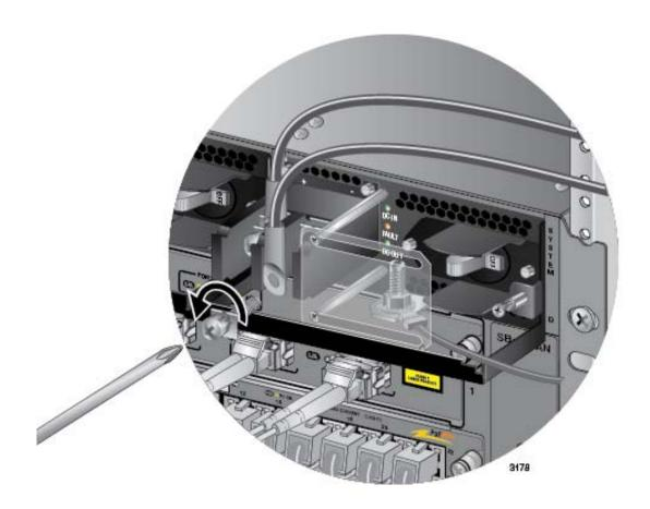
Figure 152. Removing the Negative Lead Wire
