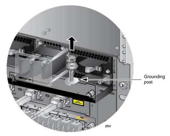
Figure 114. Removing the Nut and Washer from the Grounding Post
