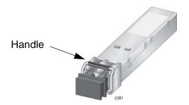
Figure 93. Handle on SFP+ Transceiver
