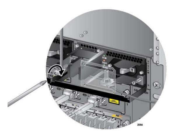
Figure 137. Connecting the Positive Wire
