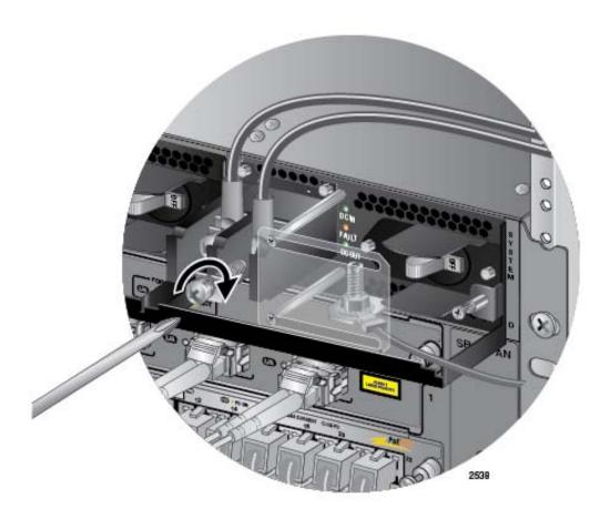
Figure 126. Connecting the Negative (-) Power Wire with a Straight Terminal
