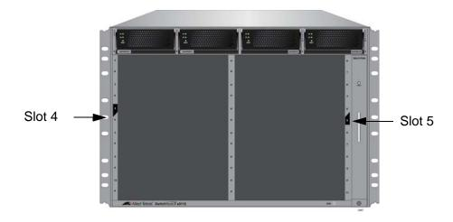
Figure 65. Slots 4 and 5 for the AT-SBx31CFC Card
