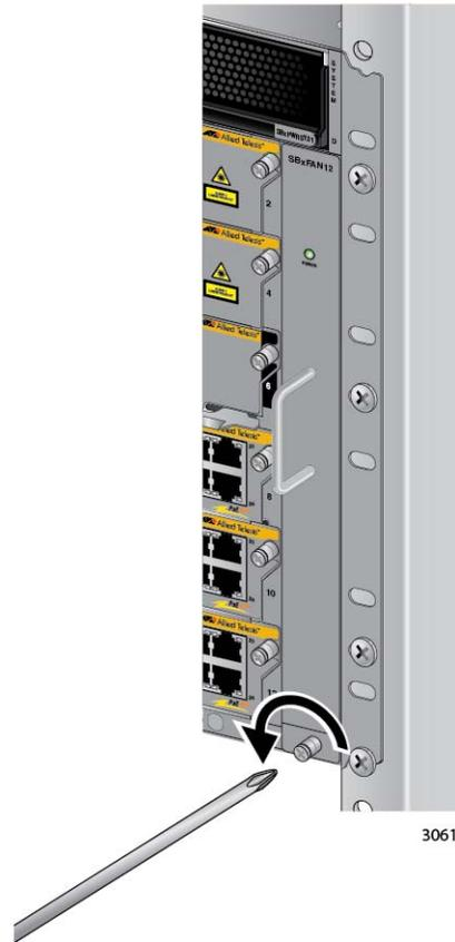
Figure 169. Loosening the Screw on the AT-SBxFAN12 Fan Module
