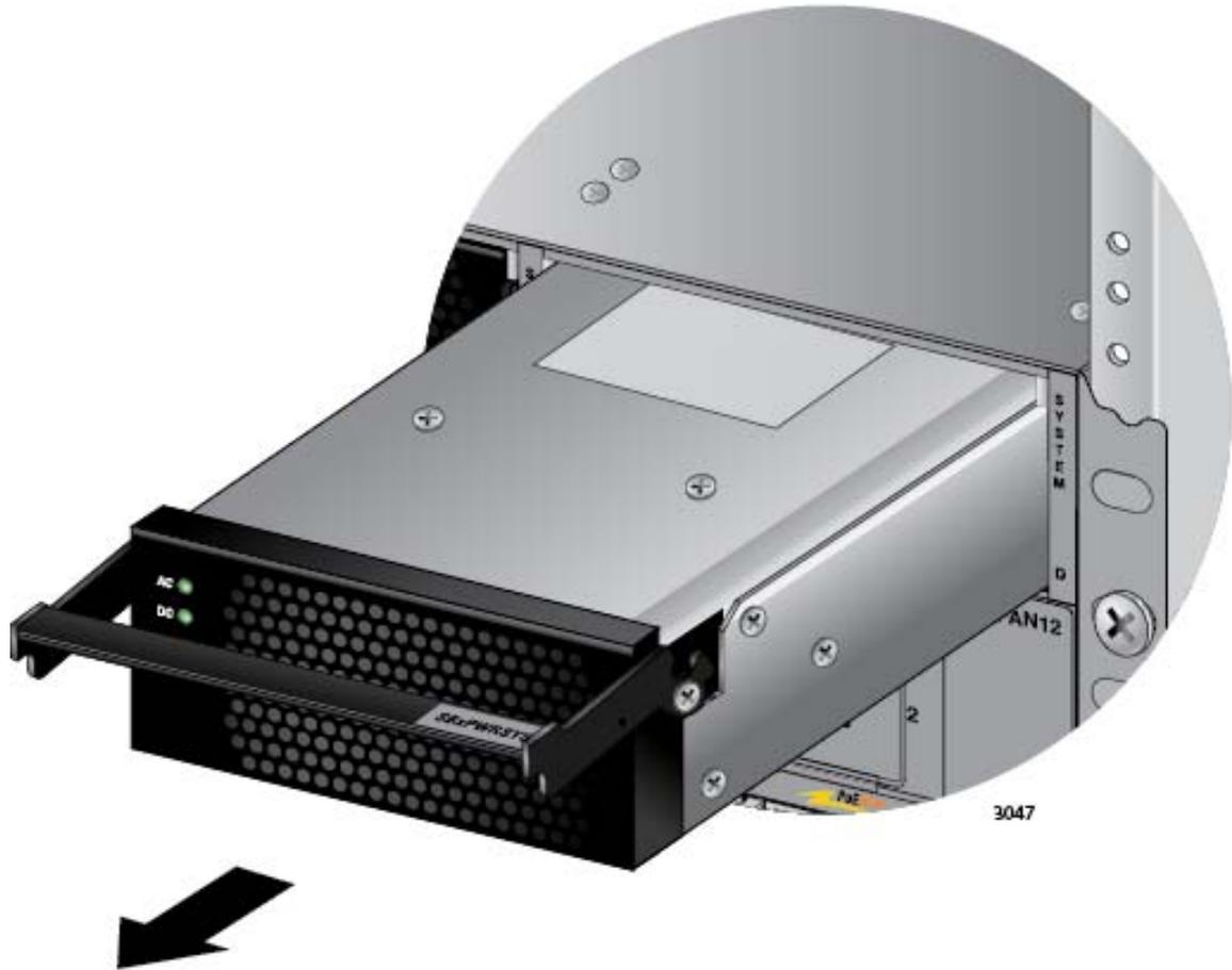
Figure 147. Removing the Power Supply from the Chassis
