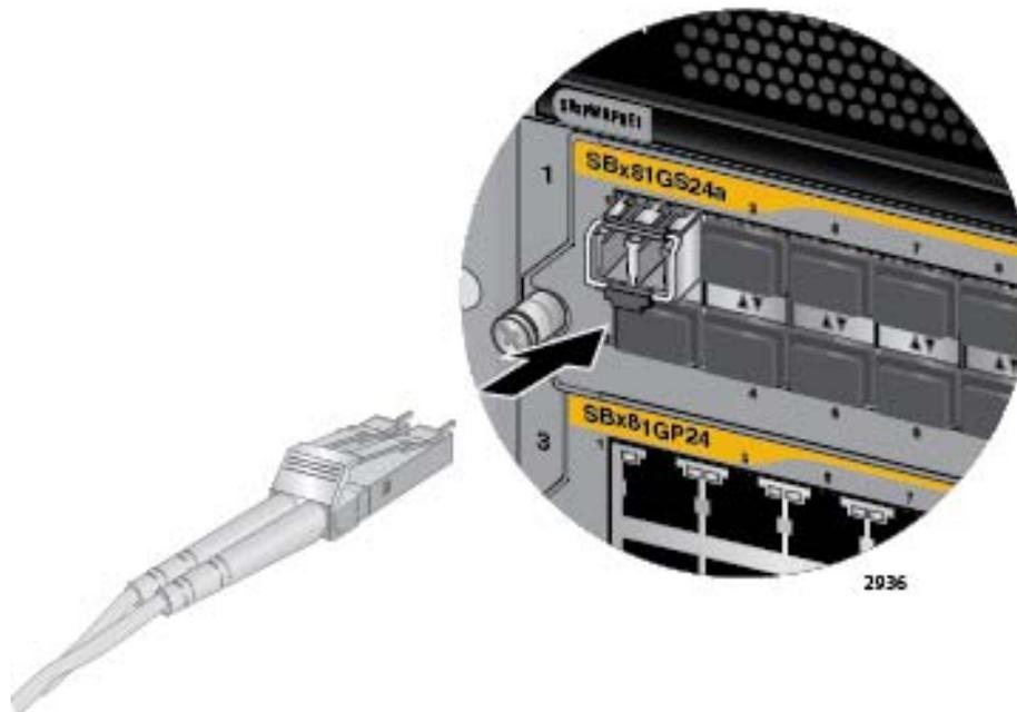
Figure 99. Attaching a Fiber Optic Cable to a Transceiver
