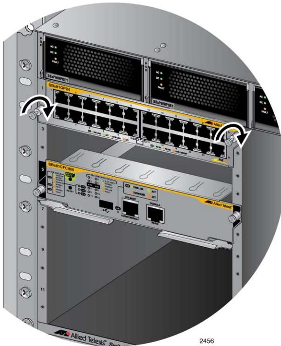
Figure 89. Tightening the Thumb Screws on an Ethernet Line Card
