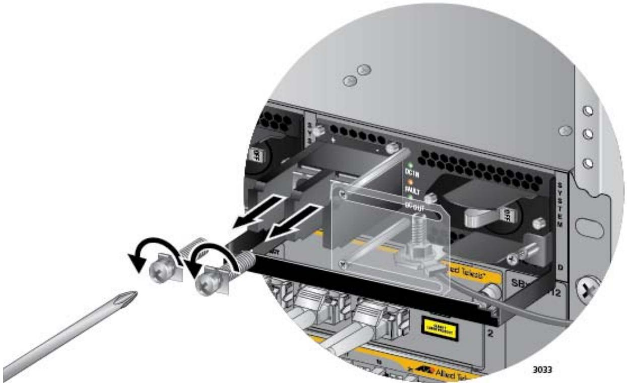
Figure 125. Removing the Terminal Screws
