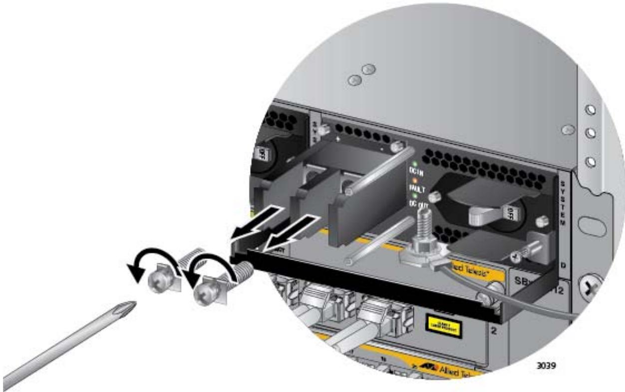
Figure 133. Removing the Terminal Screws
