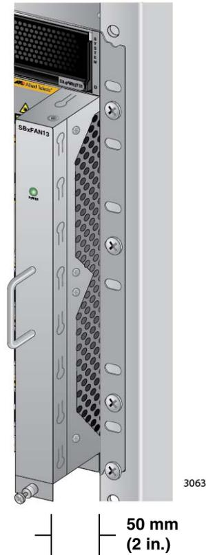
Figure 171. Withdrawing the AT-SBxFAN12 Fan Module 51 mm (2 In.) from the Chassis
