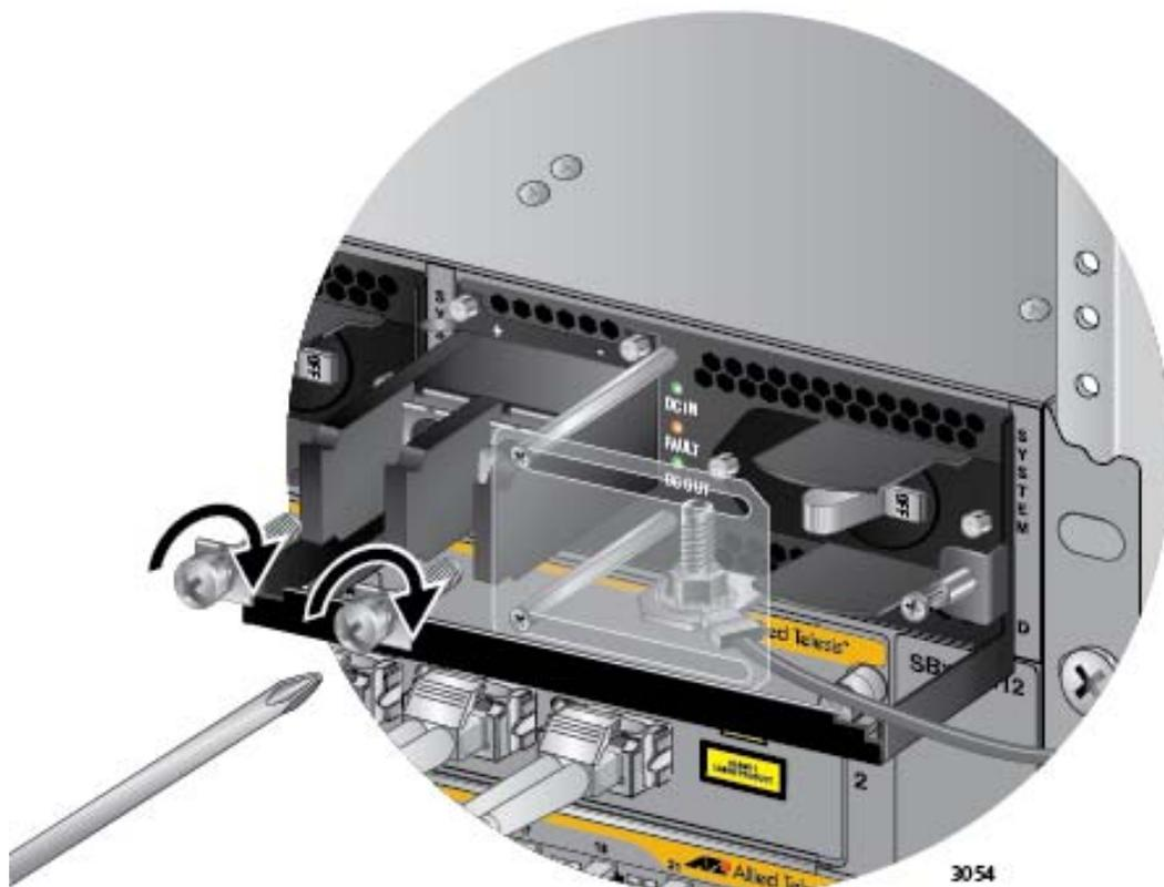
Figure 154. Reinstalling the Screws on the Positive and Negative Terminals
