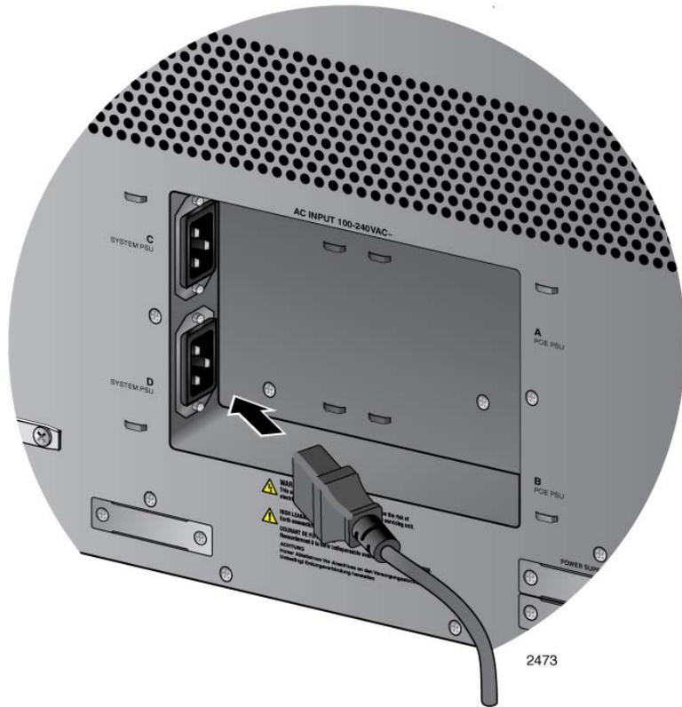
Figure 106. Connecting the AC Power Cord for the AT-SBxPWRSYS1 or AT-SBxPWRSYS2 AC System Power Supply
