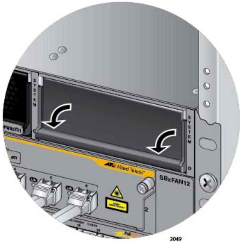
Figure 149. Lowering the Locking Handle on the Power Supply Slot Cover
