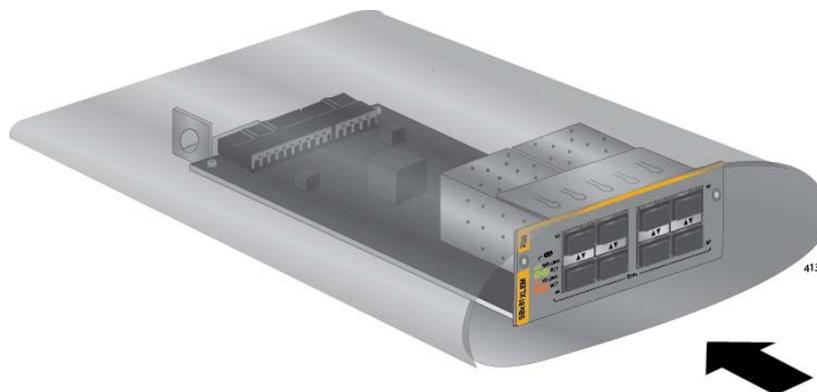
Figure 165. Storing the Expansion Module in an Anti-static Bag
