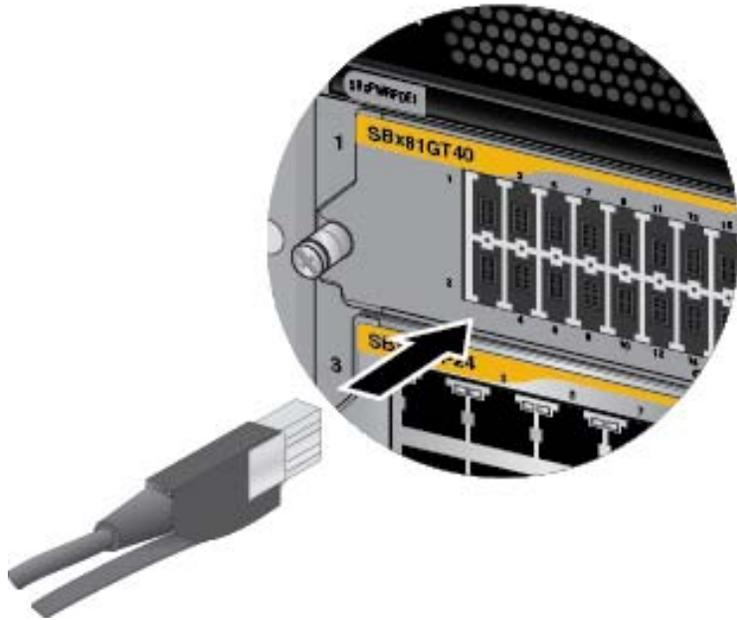
Figure 93. Connecting Cables to Ports on the AT-SBx81GT40 Line Card
