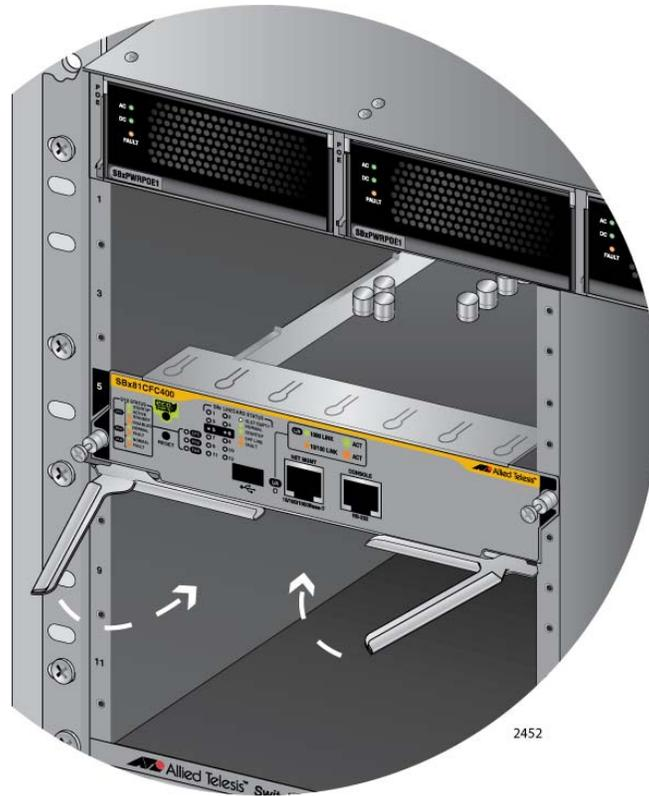
Figure 71. Closing the Locking Levers on the AT-SBx81CF400 Controller Fabric Card
