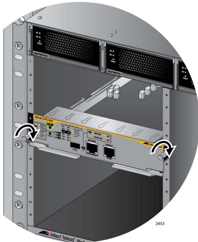
Figure 72. Tightening the Thumb Screws on the AT-SBx81CF400 Card
