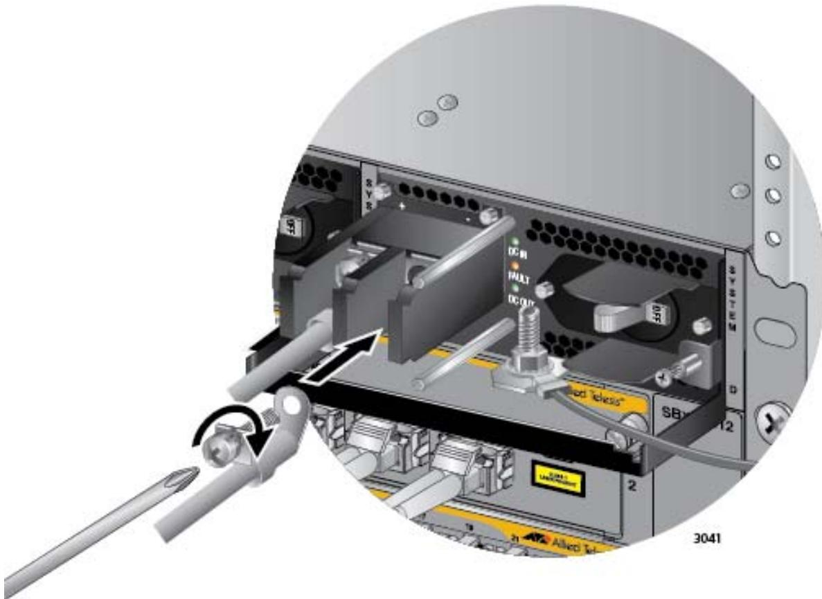
Figure 135. Connecting the Negative (-) Power Wire with a Right Angle Terminal
