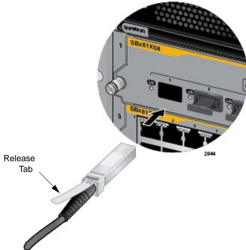
Figure 101. Installing the AT-SP10TW Cable in the AT-SBx81XS6 Line Card
