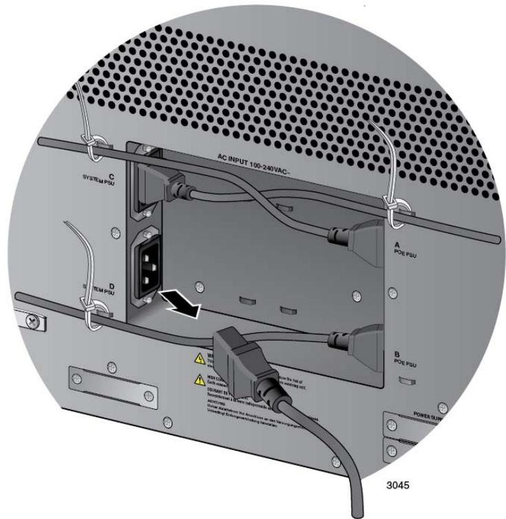
Figure 145. Disconnecting the AC Power Cord from the AC Socket on the Back Panel
