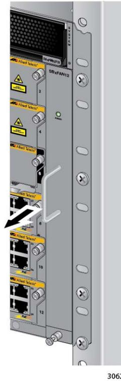
Figure 170. Loosening the AT-SBxFAN12 Fan Module from the Backplane Connector
