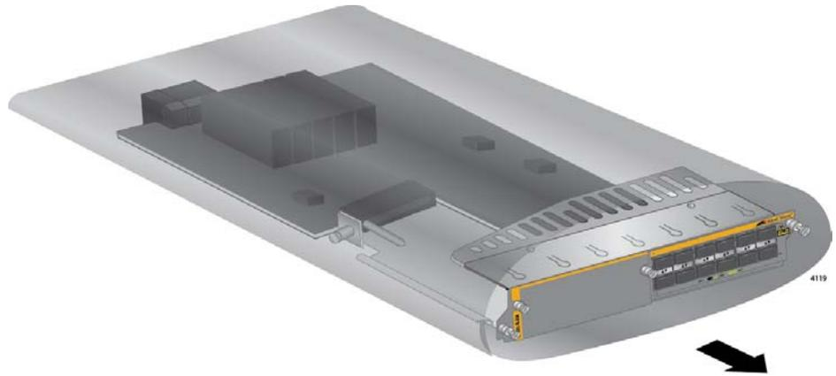
Figure 73. Removing the AT-SBx81XLEM Line Card from the Anti-static Bag
