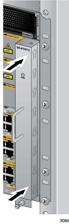
Figure 174. Securing the AT-SBxFAN12 Fan Module on the Backplane Connector
