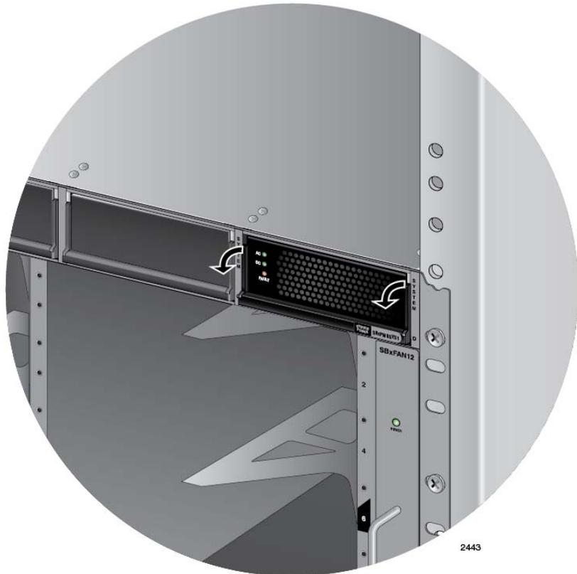
Figure 51. Lowering the Handle on the AT-SBxPWRSYS1 or AT-SBxPWRSYS2 AC System Power Supply
