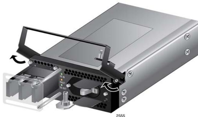
Figure 61. Raising Handle on the AT-SBxPWRSYS1 DC Power Supply
