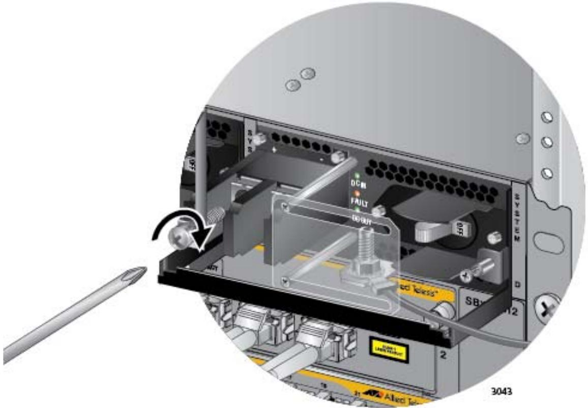
Figure 138. Connecting the Positive Wire With Bare Wire
