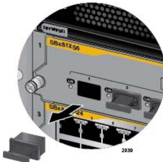
Figure 100. Removing the Dust Cover From an SFP+ Slot
