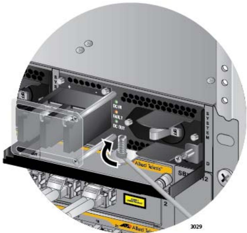
Figure 118. Attaching the Bare Grounding Wire to the Grounding Post
