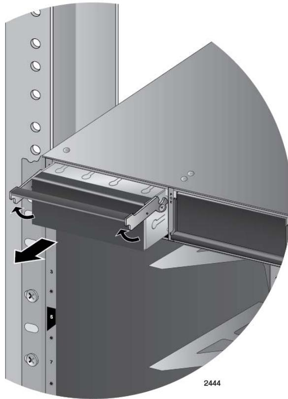
Figure 52. Removing the Blank Slot Cover from Power Supply Slot A
