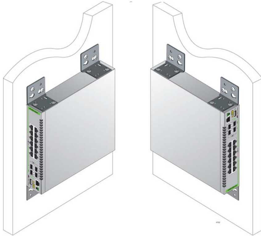
Figure 39. Positioning the Switch on the Wall
