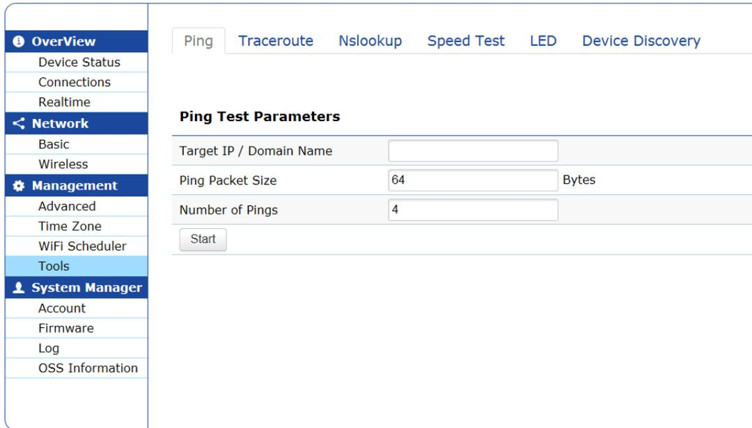
Figure 41. Ping Test Parameters Page
