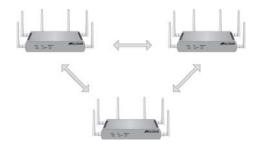
Figure 18. Invalid Loop Configuration of Access Points
