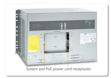
The two system and two PoE power supplies have individual power cord receptacles on the rear of the chassis, so each can be fed from separate power sources if desired to further increase reliability and resiliency. For specific power outlet requirements (dependent on voltage in your country) see the installation guide.
