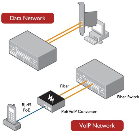
When installing two separate networks, one for data and one for voice, clients can increase the integrity of their data security by running fiber directly into the desktop with Allied Telesis Fiber NICs. In the same environment, use Allied Telesis VoIP Media Converter switches are used to get an IP phone onto fiber.
