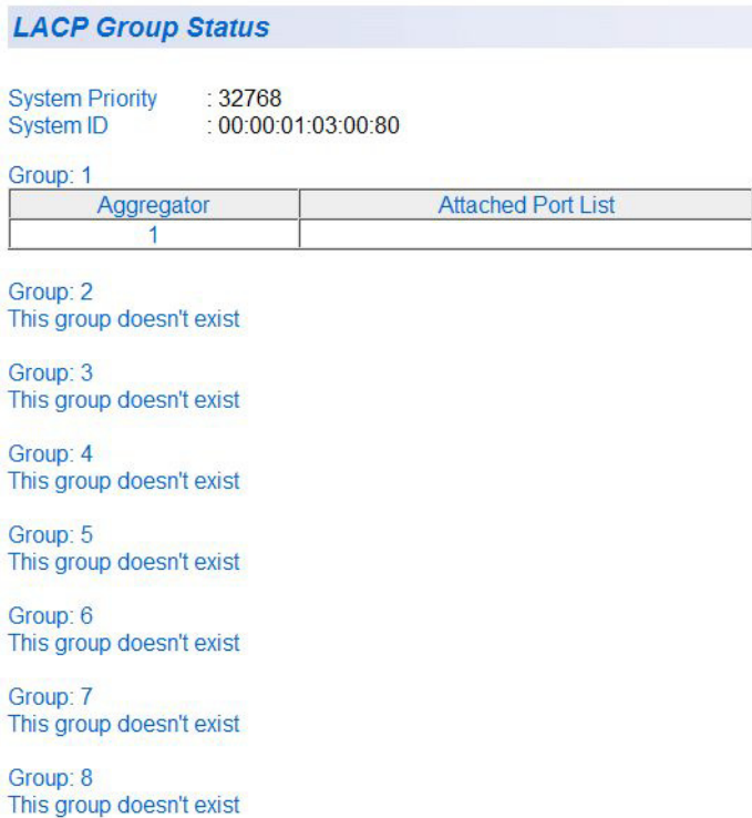
Figure 33. LACP Group Status Page with No Cables Connected
