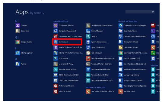
Under the "Application and Services Logs" section, select the "Allied Telesis Switch Operations" items. A log will be shown for each modification made to the switch configuration, identifying the user who made the modification and the operation performed.
