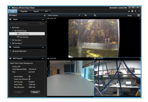
To administratively enable or disable the port, select or de-select the "Port Enabled" checkbox. To supply or remove power to the camera from the port, select or de-select the "Power over Ethernet" checkbox. Click "Apply" to apply any changes. Note that the controls will be disabled (greyed out) if the current user does not have write access to the switch, as assigned in the configuration in the **Milestone XProtect Management Client**.
