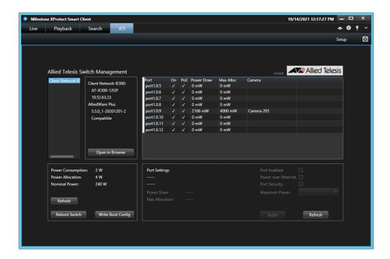
The plug-in will display information about the switch, including the hardware model and the currently running software release. It will also show a list of ports in a table at the upper right, with a summary of status information:
