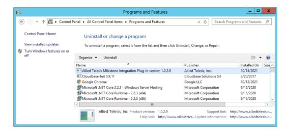
Note that any configuration in the Milestone application associated with the plug-in will **not** be removed when the plug-in is uninstalled. It is recommended that any Allied Telesis switch-related configuration be removed using the Milestone XProtect Management Client prior to uninstallation of the plug-in.
