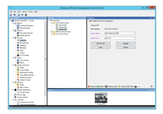
Once the desired camera association has been made, save the configuration using the save icon at the upper left, or type Ctrl-S.
