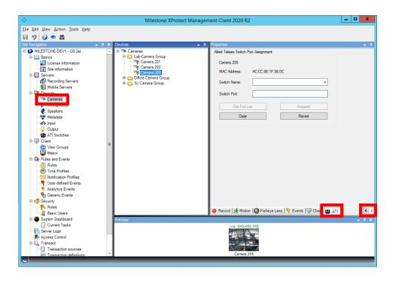
In the plug-in panel, select a switch to associate to the camera under the "Switch Name" drop-down menu. (You may also type the name of the switch into the box, in case the desired switch has not yet been configured.)
