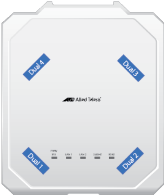
Figure 34. Antenna Axes on the TQ6602 GEN2 and TQm6602 GEN2 Access Points
