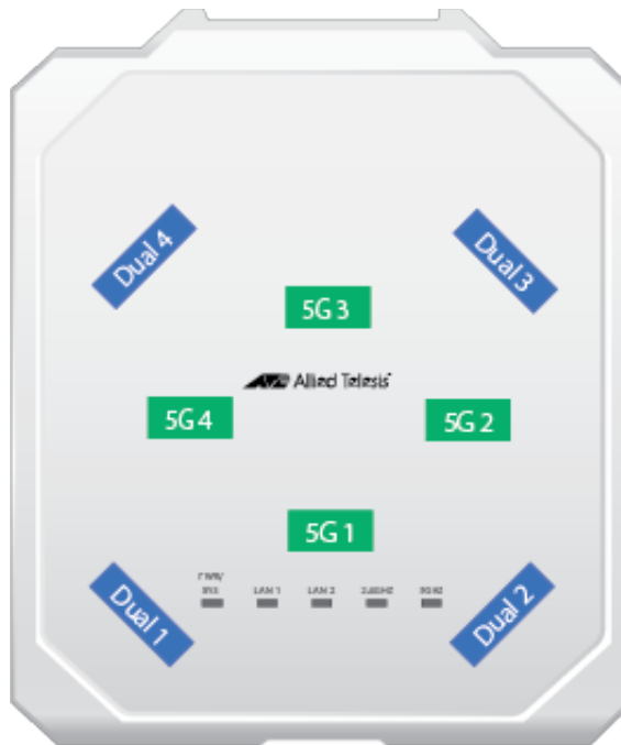
Figure 32. Antenna Axes on the TQ6702 GEN2 and TQm6702 GEN2 Access Points
