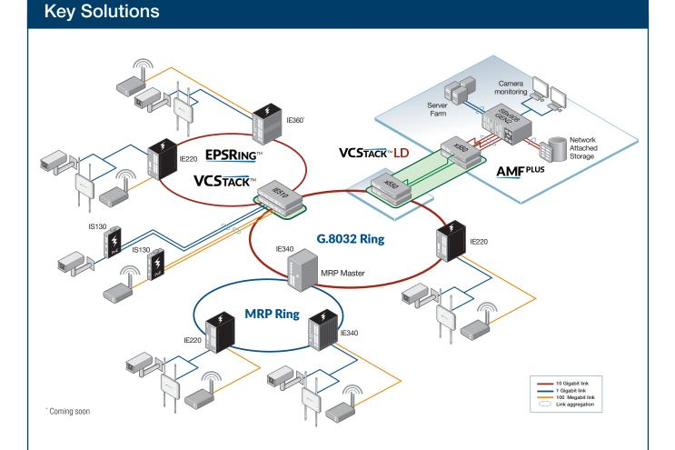
Media Redundancy Protocol (MRP), EPSRing and ERPS (ITU G.8032) provide high-speed resilient ring connectivity. This diagram shows how the IE Series can support a variety of ring network topologies.
