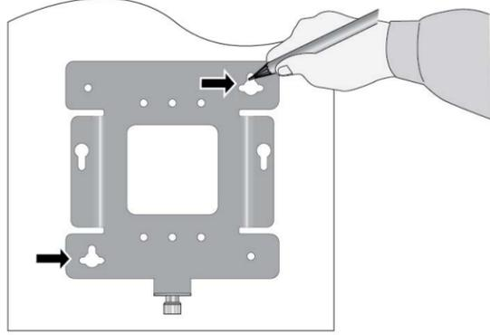
3. If necessary, pre-drill on the wall or ceiling the two marked locations of the key-hole slots for the screws.
