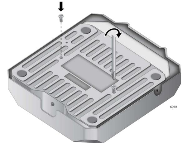
The screw collar provides the proper spacing for the mounting bracket beneath the screw head.
