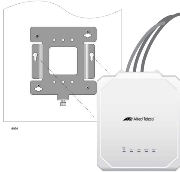
2. Slide the access point forward until its screws are seated in the bracket keyhole slots and the bracket thumbscrew is aligned with the screw hole on the front panel.
