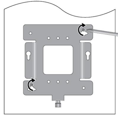
7. To secure the mounting bracket, pre-drill holes through the two bracket mounting holes opposite the key-hole slots.
