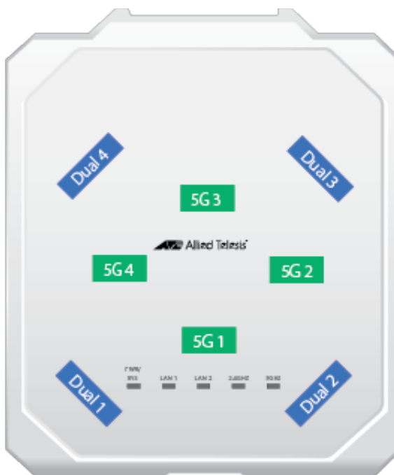
Figure 35. Antenna Axes on the TQ6702 GEN2, TQ6702 GEN2-R, and TQM6702 GEN2 Access Points
