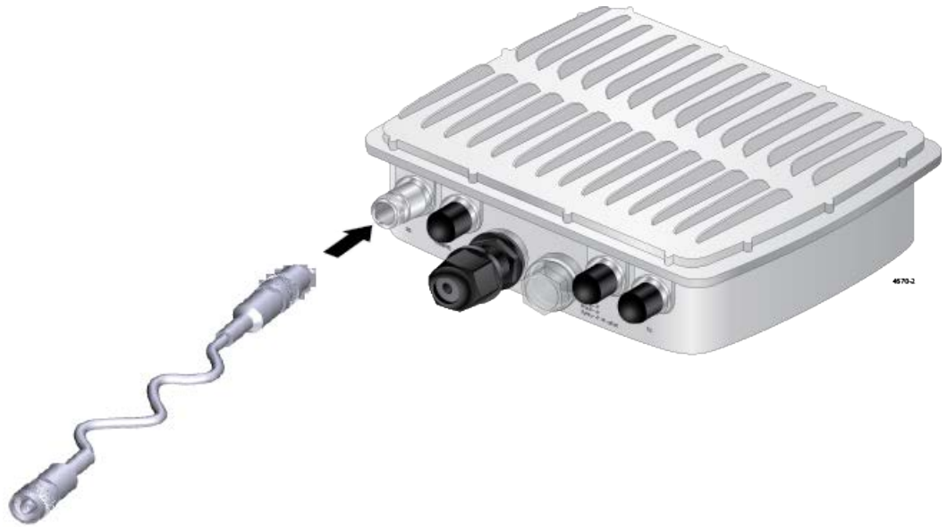
Figure 45. Attaching the cable to an Antenna Connector
