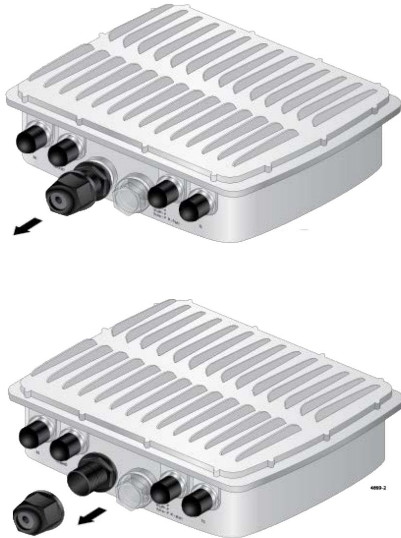
Figure 11. Removing the Cap from the LAN Port
