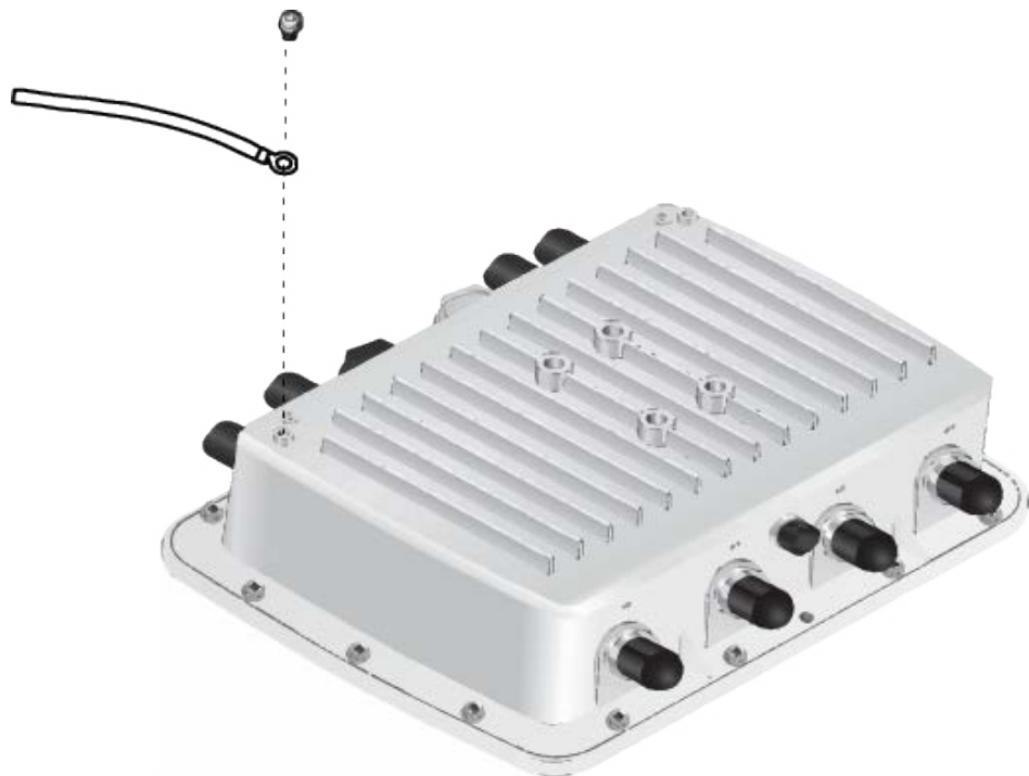
Figure 10. Connecting the Ground Wire to the Access Point
