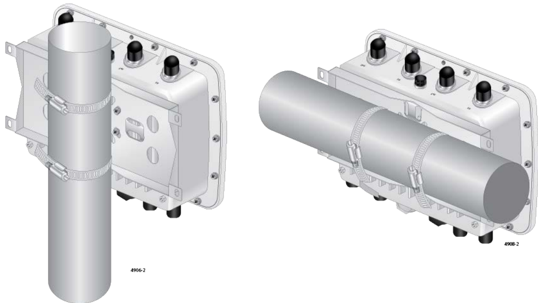
Figure 31. Pole Orientations for the Access Point
