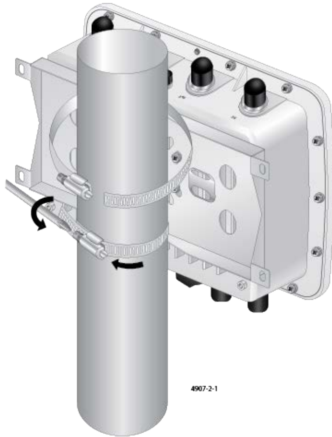
Figure 36. Inserting the Strap Ends into the Screws
