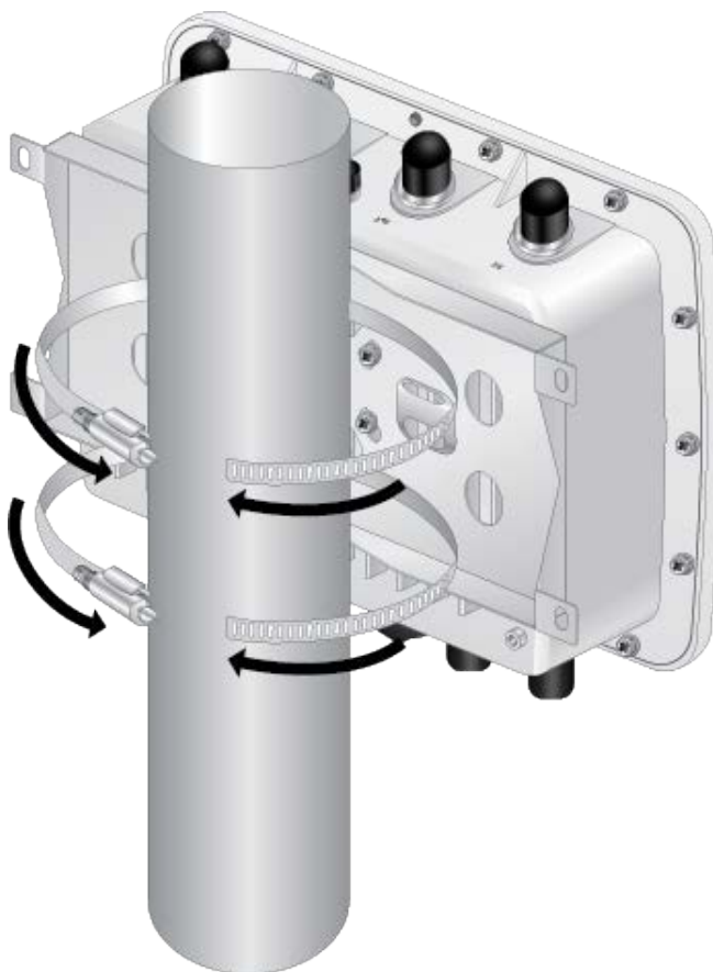
Figure 35. Wrapping the Pole Straps Around the Pole
