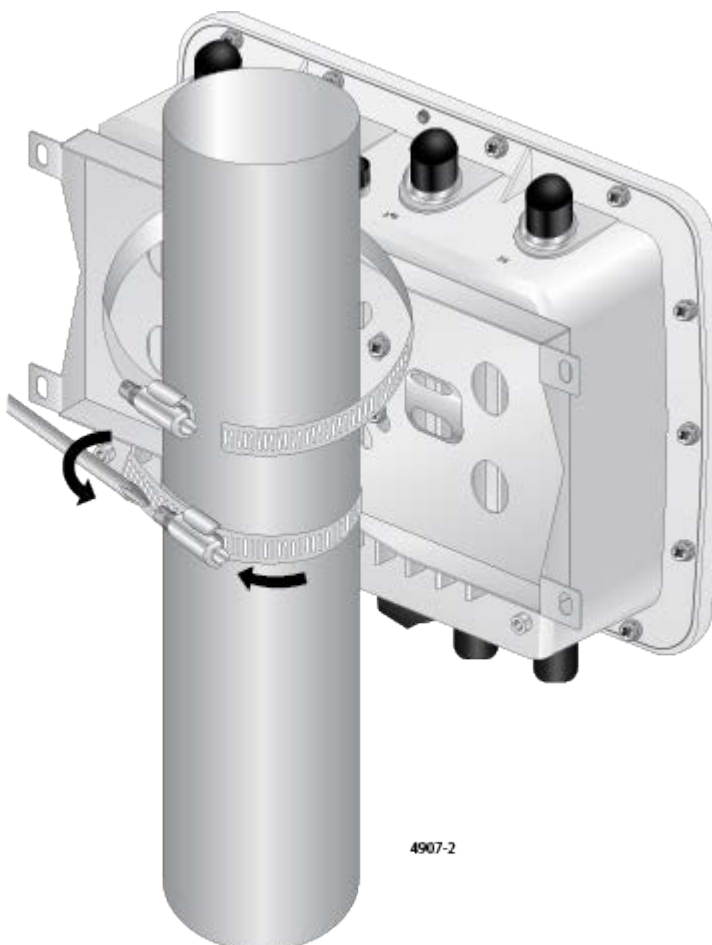
Figure 37. Tightening the Straps
