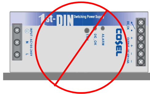
Figure 7. Unsupported Table, Desk, or Shelf Installation
