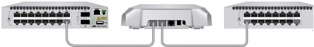
Figure 30. PORT2 in Cascade Mode with a Networking Device
