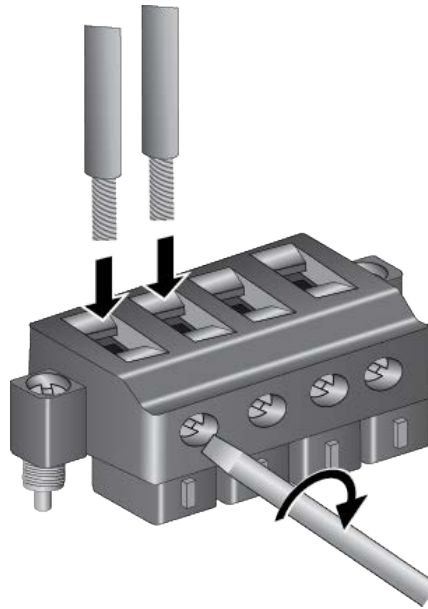
Figure 58. Inserting DC Wires into the POWER Plug
