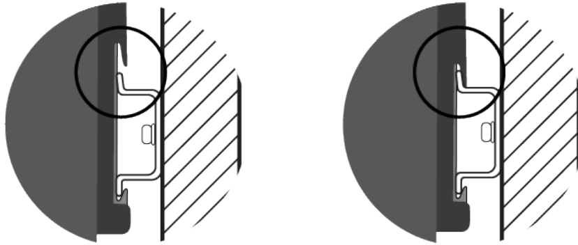
Figure 20. Installing the Switch on a DIN Rail - 3
