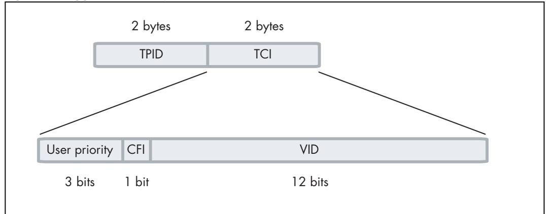
**TPID** is the tag protocol identifier, which indicates that a tag header is following and contains the user priority, Canonical Format Indicator (CFI), and the VLAN ID.
