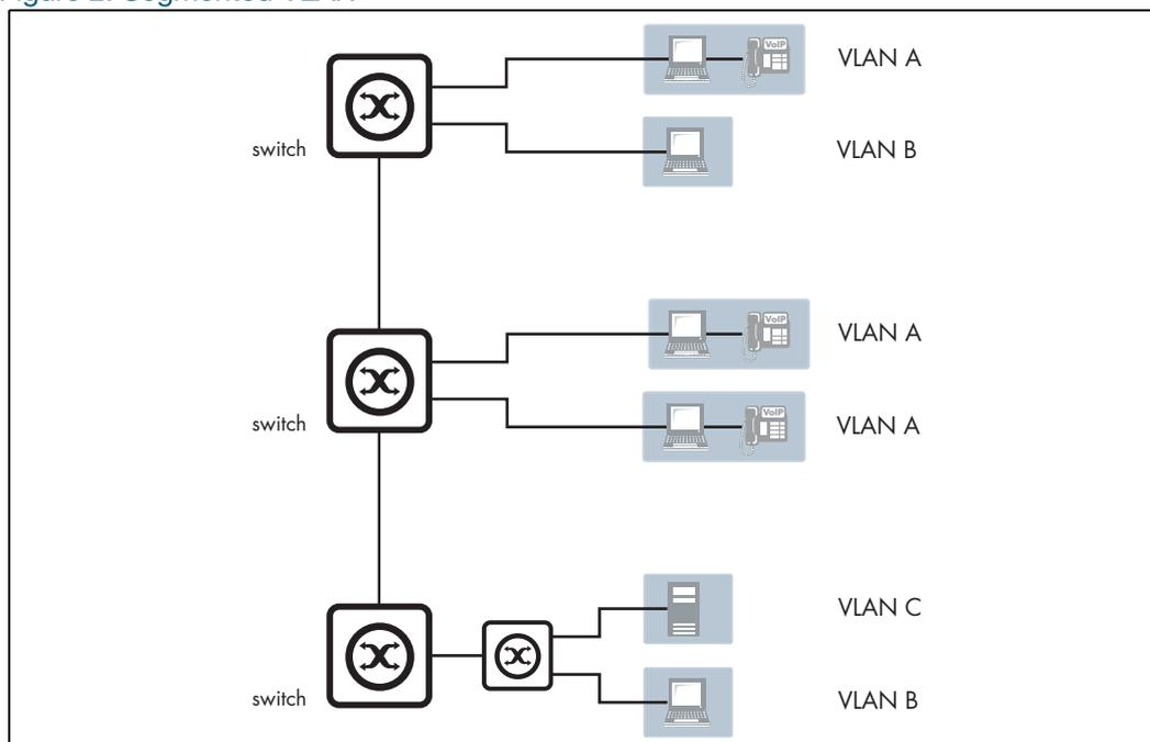
Instead of the LANs corresponding to physical areas divided from each other by routers, there are virtual LANs distributed across the network. For example, all the devices in the various areas labeled “LAN A” all belong to a single virtual LAN—i.e. a single broadcast domain.
