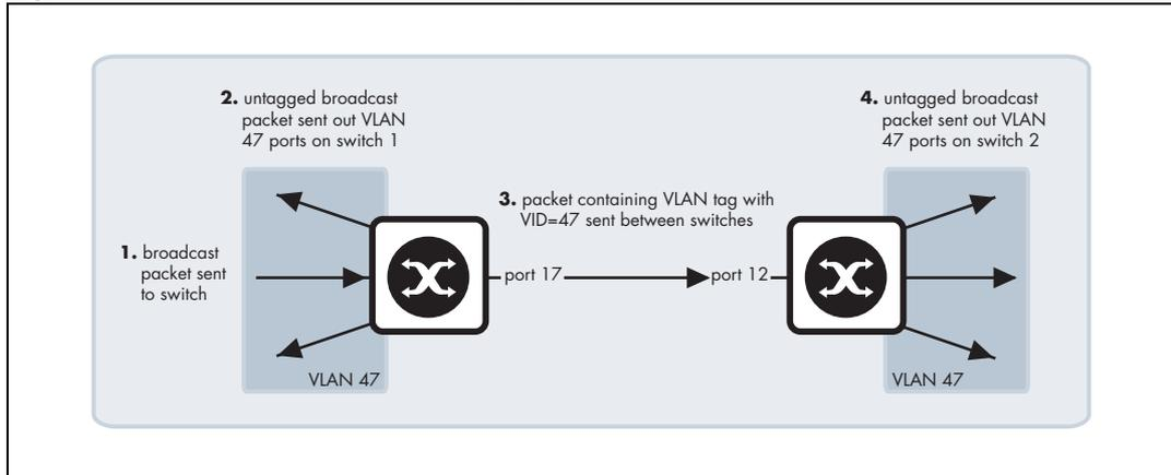
The tag makes it very easy for the second switch to know what to do with the packet, because the tag marks this packet as belonging to VLAN 47, and switch 2 knows exactly what it should do with packets that belong to VLAN 47.
